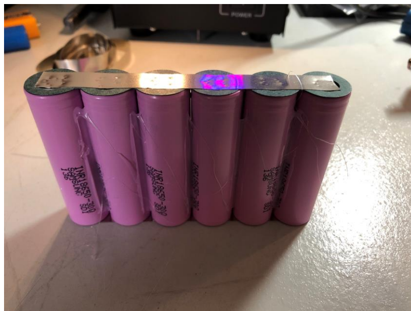
Figure 42: Six cells welded together to form a brick
