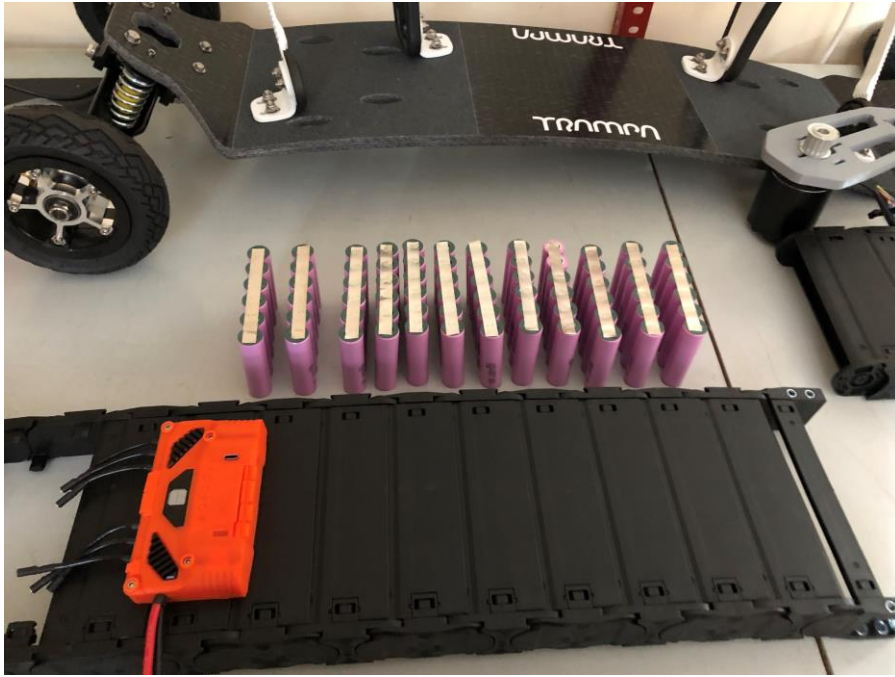
Figure 43: All 12 bricks spot welded and ready for installation
