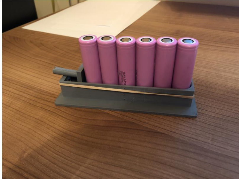
Figure 41: Group of 6 18650 cells ready for welding
