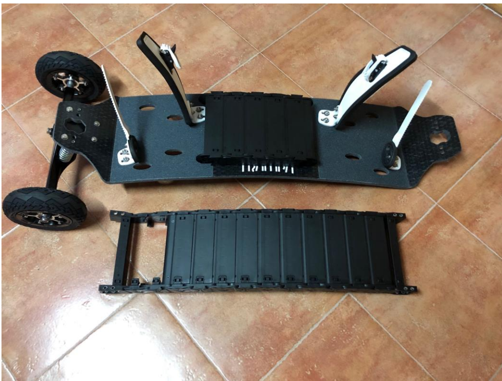
Figure 40: Cable chain design as a battery pack enclosure
