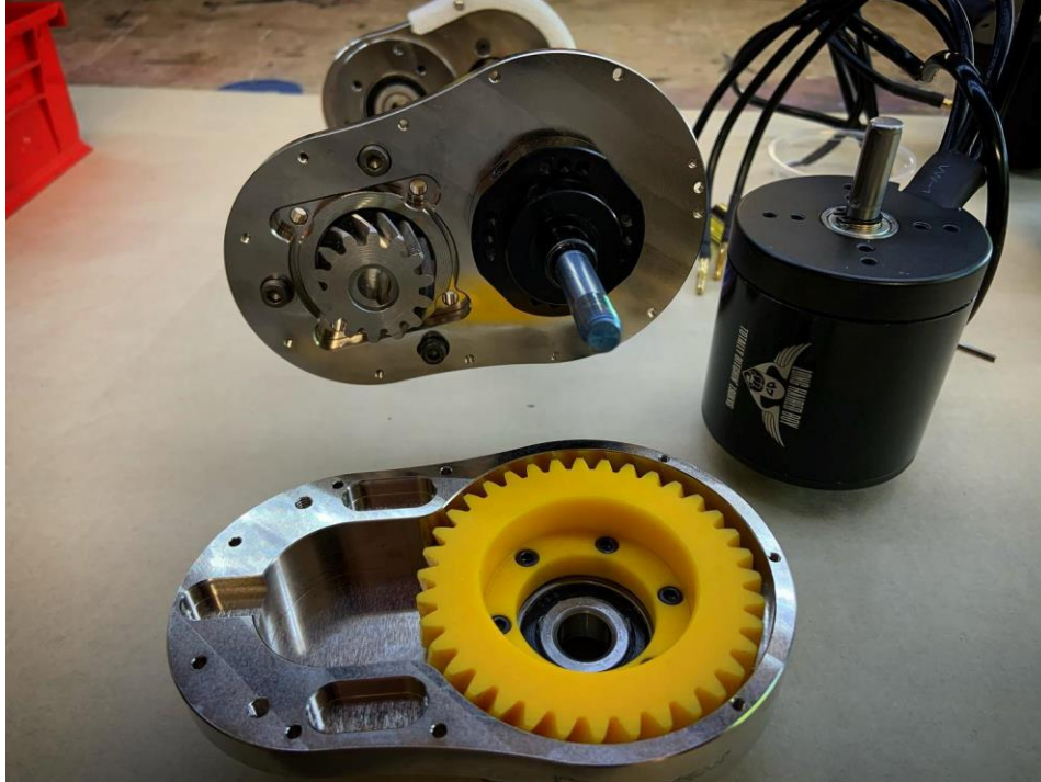
Figure 30: Helical gear drivetrain assembly from an e-longboard
