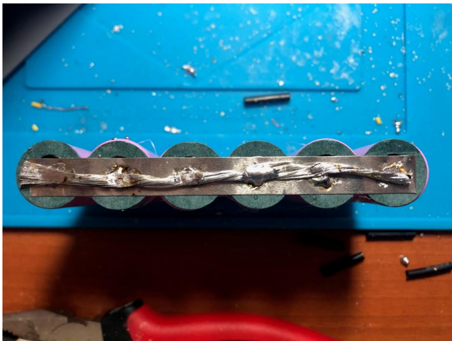
Figure 44: Copper cable welded on top of nickel strip
